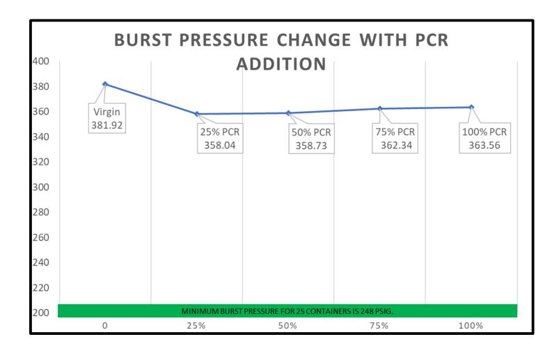
No failures to the container occurred during the PARG 10.0 testing below the minimum for the DOT-2S requirement of 248 psig (17.1bar).
