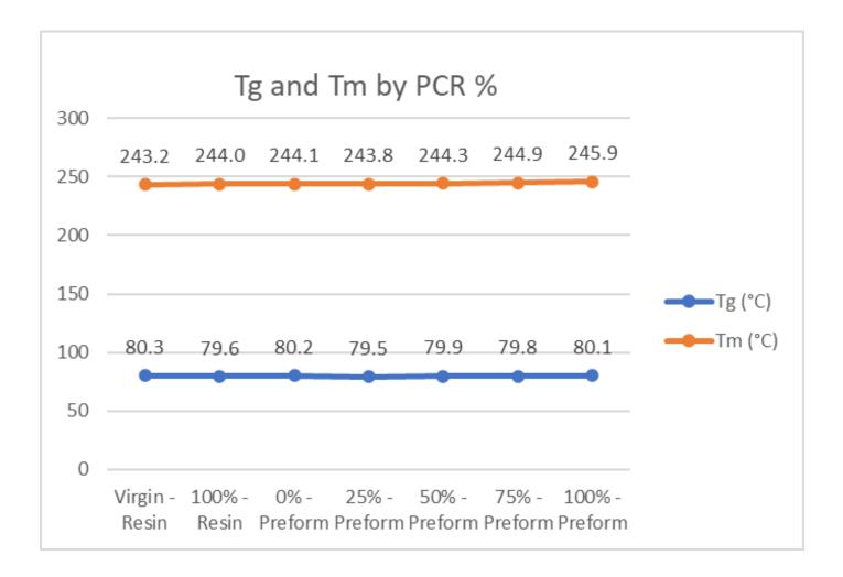
**Tg** describes how amorphous plastics or the amorphous portion of semi-crystalline plastics transition from a rigid, glass-like state to a more flexible, rubbery state.
